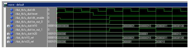
After the assertion of clk\_enable (replicated by ce\_out\_0), a new value is computed and output to ST10 for every cycle of the base rate clock.
