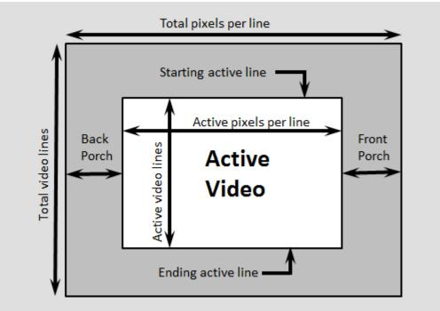
This figure shows a video frame with the horizontal porch split into a front and a back porch.
