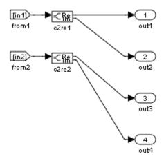
The model maintains the separation of real and imaginary components throughout the cosimulation path. The Compare subsystem performs separate comparisons and separate scope displays for the real and imaginary signal components.
