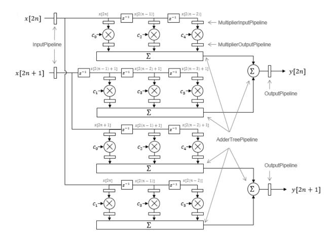
For symmetric or antisymmetric coefficients, the filter architecture reuses the coefficient multipliers and adds design delay between the multiplier and summation stages as required.
