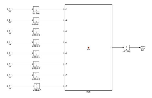
The following shows a chain of multiplications as coded in the  $\verb|mult8|$  MATLAB Function block:
