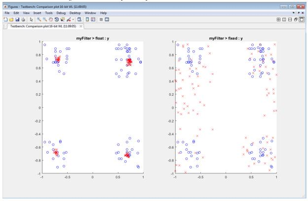
The plot shows that the fixed-point results do not closely match the floating-point results.
