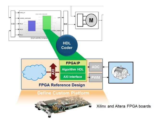
Use the HDL Coder generated AXI4-Lite interface to connect the IP core with an AXI4 or AXI4-Lite Master device such as:
