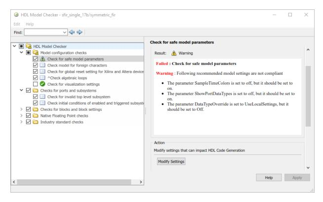
To apply the correct model configuration settings that the Model Checker reported in the **Result** subpane, click the **Modify Settings** button. After you click **Modify Settings**, the **Result** subpane reports the changes that were applied. You can now run this check.
