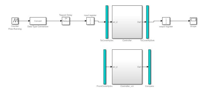
The lower section of the validation model contains a copy of the original DUT (Controller\_vnl). This single-rate subsystem runs at its original rate.
