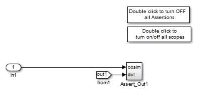
For each output of the DUT, HDL Coder generates an assertion checking subsystem (Assert\_OutN). The subsystem computes the difference (err) between the original DUT output (dut ref) and the corresponding cosimulation output (cosim). The subsystem routes the comparison result to an Assertion block. If the comparison result is not zero, the Assertion block reports the discrepancy.
