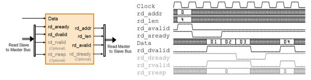
The DUT waits for rd\_aready to become high to initiate a read request. When rd\_aready is high, the DUT can send out the read request. The read request consists of the rd\_addr, rd\_len, and rd\_avalid signals of the Read Master to Slave bus. The slave IP or the external memory responds to the read request by sending the Data at
