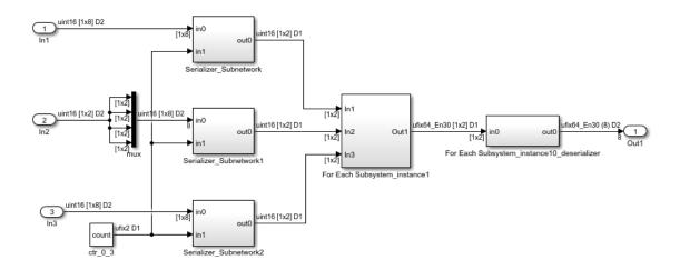
If you double-click the For Each Subsystem\_Instance1 block, you see the algorithm computed for the size 2 subarrays of inputs In1 and In3.
