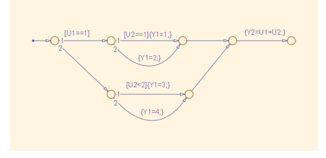
The following generated VHDL code excerpt shows the nested IF-ELSE statements obtained from the flow diagram.
