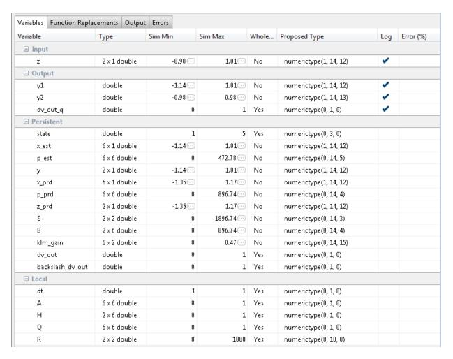
Examine the types proposed in the above table for variables instrumented in the top-level design.
