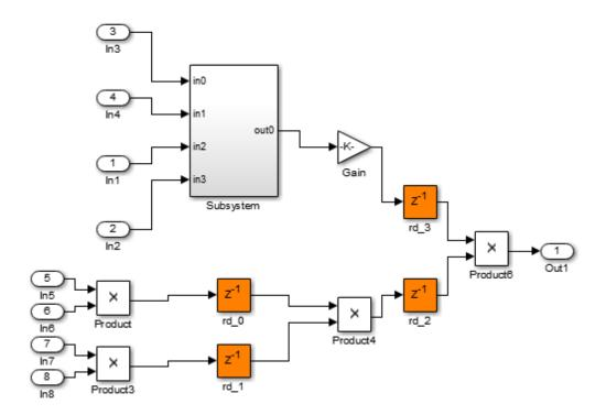
The subsystem now contains pipeline registers:
