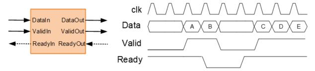
For example, if you have a FIFO in your DUT to store a frame of data, to apply back pressure to the upstream component, you can model the Ready signal based on the FIFO Full signal.
