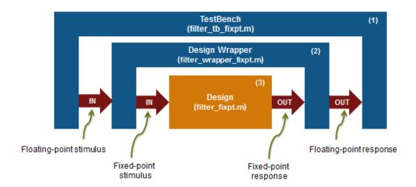
The following steps are performed during fixed-point type validation process:
