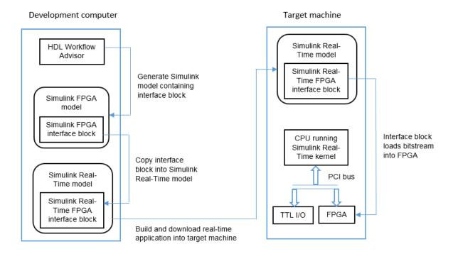
To learn more about the workflow, see "FPGA Programming and Configuration" (Simulink Real-Time).
