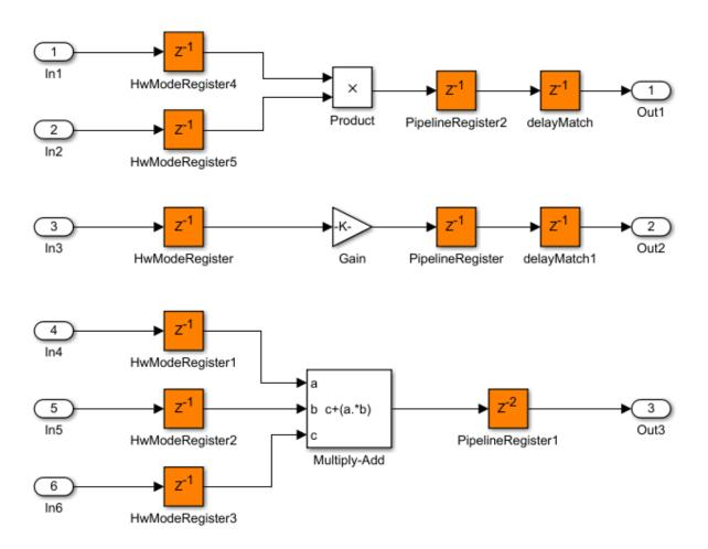
The blocks have a different number of pipeline registers at the output ports. To match the delays, HDL Coder adds a delay at the output of the Product and Gain blocks.
