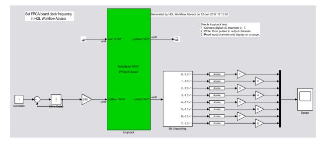
This generated model contains a masked subsystem with the same name as the subsystem in the Simulink FPGA domain model. Although the appearance is similar, this subsystem does not contain the Simulink algorithm. Instead, the algorithm is implemented in an FPGA bitstream. You reference and load this algorithm into the FPGA from this subsystem.
