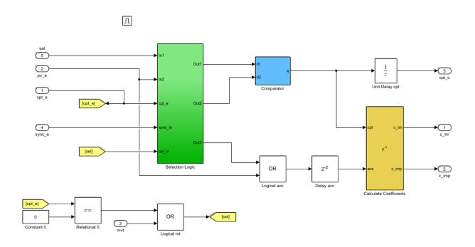
To debug internal signals in this model, mark them as test points. For example, you can designate the output signal from the Logical acc block that performs the OR operation as a test point.
