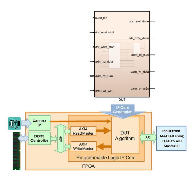
You can model your algorithm with Data and AXI4 Master protocol signals at the DUT ports and then map the signals to AXI4 Master interfaces. To learn how to model your DUT algorithm for AXI4 Master interface mapping, open this Simulink™ model. The DUT Subsystem contains a simple algorithm that reads data from the DDR and writes back to a different address in the DDR memory.
