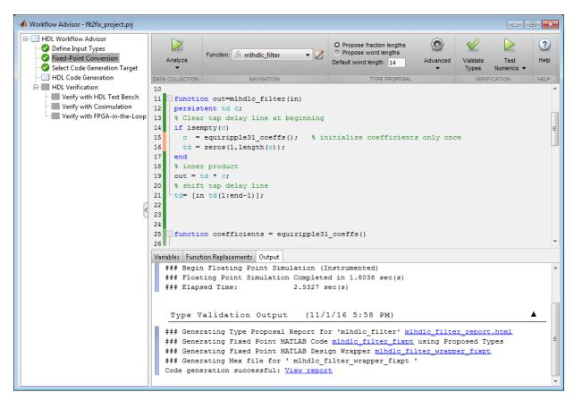
Click the links to the generated code in the Workflow Advisor log window to examine the generated fixed-point design, wrapper, and test bench.
