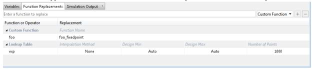
You can add and remove function replacements from this list. If you enter a function replacements for a function, the replacement function is used when you build the project. If you do not enter a replacement, the tool uses the type specified in the original MATLAB code for the function.
