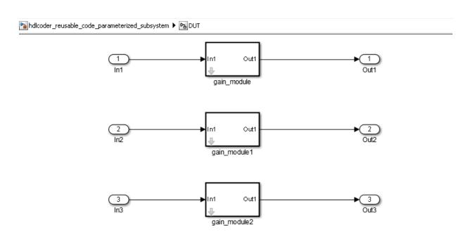
In hdlcoder\_reusable\_code\_parameterized\_subsystem/DUT, the gain modules are subsystems with gain values represented by tunable mask parameters. Gain values are: 4 for gain\_module, 5 for gain\_module1, and 7 for gain\_module2.
