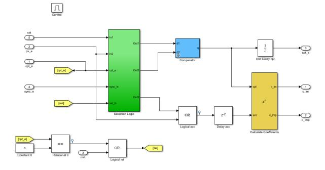
The model has three additional test points. These test points are inside the Selection Logic subsystem, the Comparator Subsystem, and the Calculate Coefficients Subsystem blocks.
