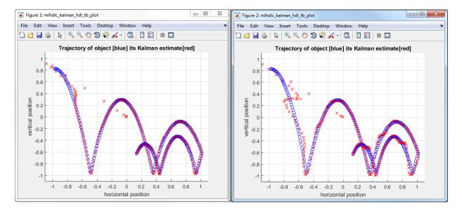
Having chosen comparison plots option you will see additional plots that compare the floating and fixed point simulation results for each output variable.
