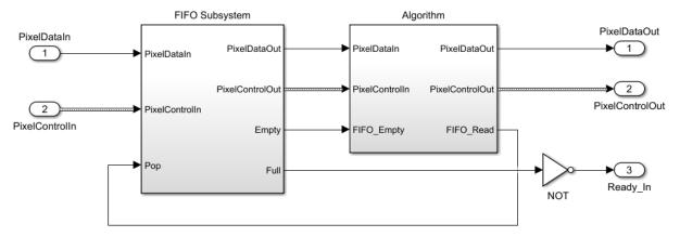
The **FIFO Subsystem** block uses HDL FIFO blocks for the **Pixel Data** and for the **Pixel Control Bus** signals.
