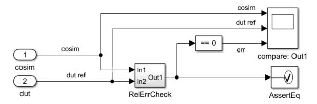
RelerrCheck has a MATLAB Function block that shows how HDL Coder accounts for the relative error when checking for numerical accuracy.
