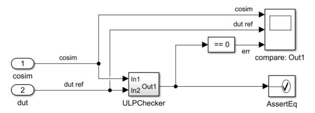
The ULPChecker has a MATLAB Function block that shows how HDL Coder accounts for the ULP error when checking for numerical accuracy.
