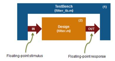
For floating-point to fixed-point conversion, the following requirements apply to the original design and the testbench:
