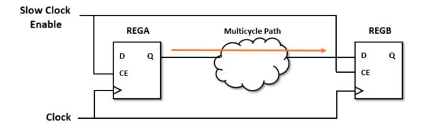
This figure shows a multicycle path that takes a certain number of clock cycles, say N, for the data to progagate from REGA to REGB. By default, the synthesis tools define the setup edge at the next active clock edge and the hold edge at the same active clock edge with respect to the destination clock signal. For a multicycle path that takes N clock cycles, the constraints redefine the setup and hold edge to allow for the longer data propagation time.
