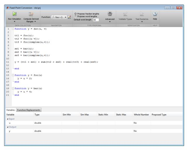
In the generated fixed-point code, the number of each fixed-point specialization matches the number in the Source Code list which makes it easy to trace between the floating-point and fixed-point versions of your code. For example, the generated fixed-point function for foo > 1 is named foo s1.
