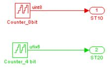
As shown in the next figure, the outputs of the multirate DUT drive To Workspace blocks in the test bench. These blocks inherit the sample times of the DUT outputs.
