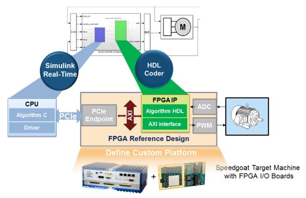
HDL Coder supports the Speedgoat IO333-325K board with the Simulink Real-Time FPGA I/O workflow. This workflow uses the IP Core Generation workflow infrastructure and has these key features:
