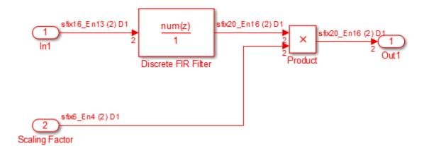
The subsystem contains a Discrete FIR Filter block and a constant multiplier. The multiplier is included to show the optimizations operating over all eligible logic in a subsystem.
