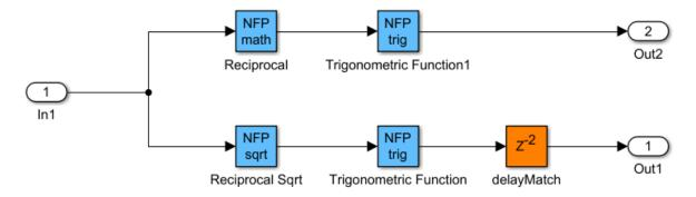
In the generated model, you see that the code generator adds a latency for each floating-point operator and adds a matching delay of length 2 to balance both paths. The operator latency is equal to the **Delay length** of the Delay block inside the side that NFP block. and then see the delay length of the Delay block. For example, if you double-click the NFP
