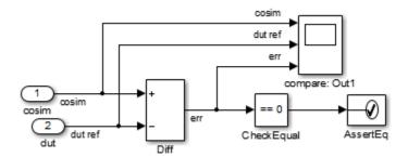
This subsystem also routes the dut ref, cosim, and err signals to a Scope for display at the top level of the model.
