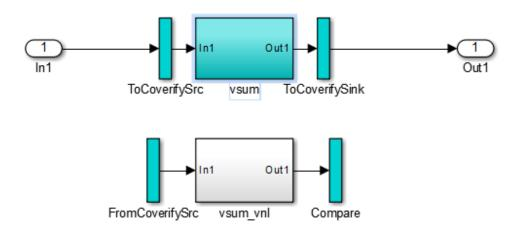
The vsum subsystem has been highlighted in cyan. This highlighting indicates that the subsystem differs in some respect from the vsum subsystem of the original model.
