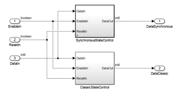
• If you double-click the **SynchronousStateControl** subsystem, a badge **S** is displayed in the Simulink editor to indicate that blocks inside the subsystem are using synchronous hardware semantics.
