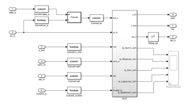
In the generated model, you see the test points at the DUT output ports connected to a TestPointScope block that is commented out. To observe the simulation results for these signals, uncomment the Scope block, and then run the simulation.
