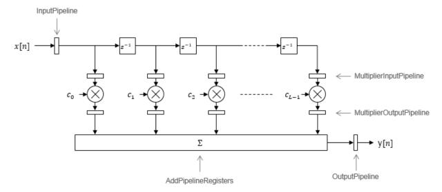
By default, the block implements linear adder logic. When you enable AddPipelineRegisters, the adder logic is implemented as a pipelined adder tree. The adder tree uses full-precision data types. If you generate a validation model, you must use full precision in the original model to avoid validation mismatches.
