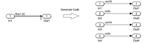
In the generated code, the array of bus expansion results in four scalar signals at the input and output ports. For the first bus object, the input ports are  $In_1_a$  and  $In_1_b$ . For the second bus object, they are  $In_2_a$  and  $In_2_b$ . At the output, for the first bus object, they are  $Out_1_a$  and  $Out_1_b$ . For the second bus object, they are  $Out_2_a$  and  $Out_2_b$ .
